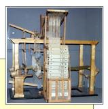
with such complex patterns as brocade, damask and matelassé. It was invented by Joseph Marie Jacquard in 1804. The loom was controlled by a "chain of cards", a number of punched cards, laced together into a continuous sequence.
